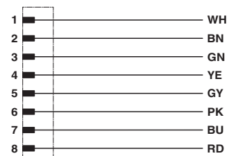
Contact assignment of the M12 plug and the M12 socket
